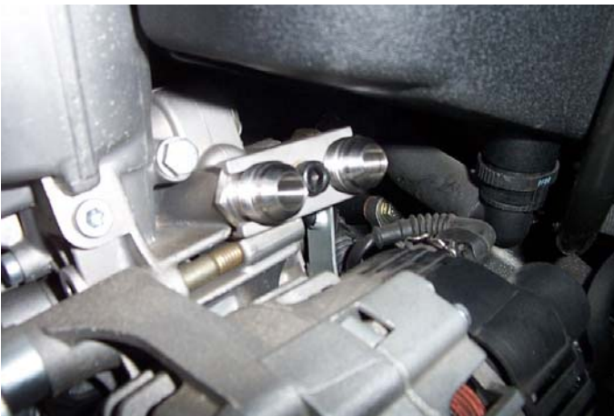
Fittings installed on housing with no hose
